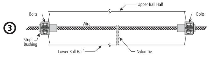
Put the upper ball half in place and install four 5/16" X 1" nylon bolts, nuts, and two flat washers per bolt, into the holes and torque to 26 inch-pounds.
