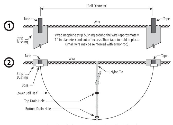
Thread the 24" nylon tie through the two bottom drain holes and secure to the wire. This should hold the lower half in place while the upper half is being installed. You may remove or leave the nylon tie after installation.
